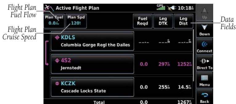
Flight Plan Fuel Flow and Cruise Speed on Active Flight Plan Page
