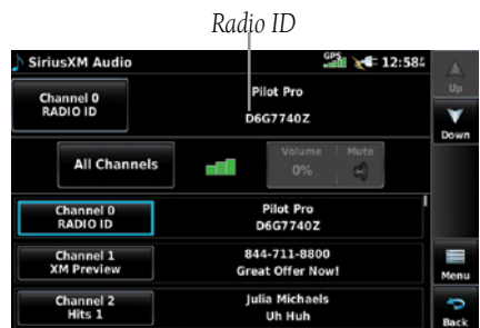
Accessing the SiriusXM Radio ID (Channel 0)
